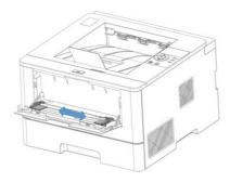
3. Load the paper into the manual feed tray with the printing side up. When using letterhead paper or preprinted paper, load the paper in the correct direction as shown in the illustration.
