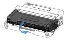
Make sure the toner cartridge is properly loaded, otherwise it may deviate from the drum.
