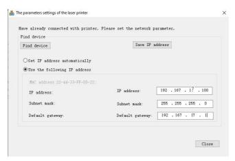
(2) Select "Use the IP address below" to set the static IP. The default static IP address is "192.167.100", the default subnet mask is "255.255.255.0", and the default gateway is "192.167.17.1". Click "Save network parameter settings" to save and write the current static IP of the printer.
